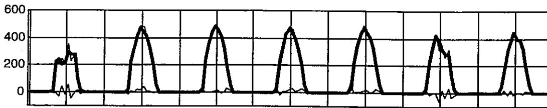
Figure 8 The diagram show the measured (heavy line) and the predicted (fine line) output power of the collector loop as well as the residuals (fine line) [ \text{W/m}^2 ]. The diagram covers the periods 92-06-06--12.
